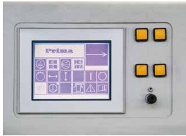
Touch screen for adjustment and drive of printing heads
